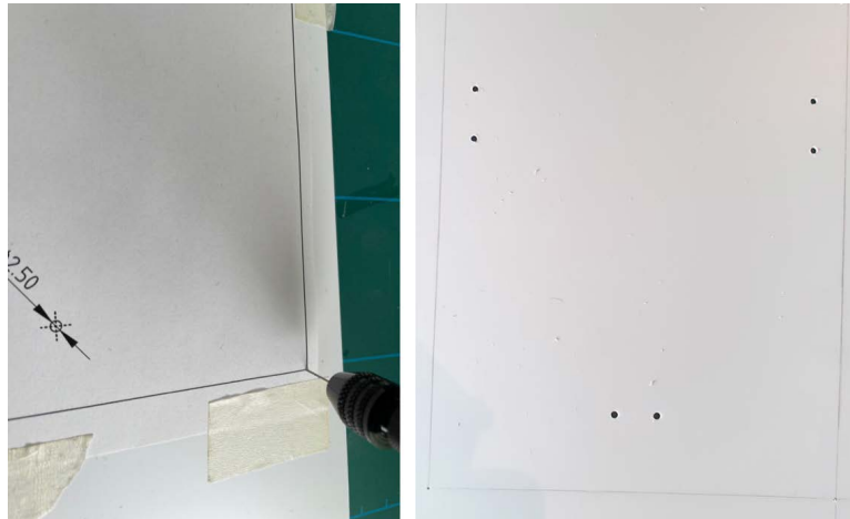
Figure 4.2 – Marking the plastic with dots
