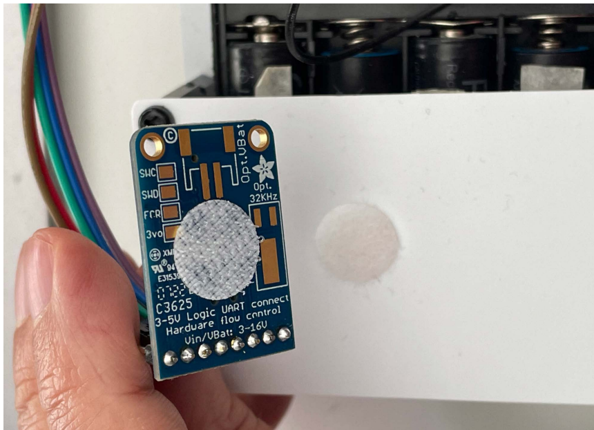
Figure 9.4 – Bluefruit module Velcro connection
