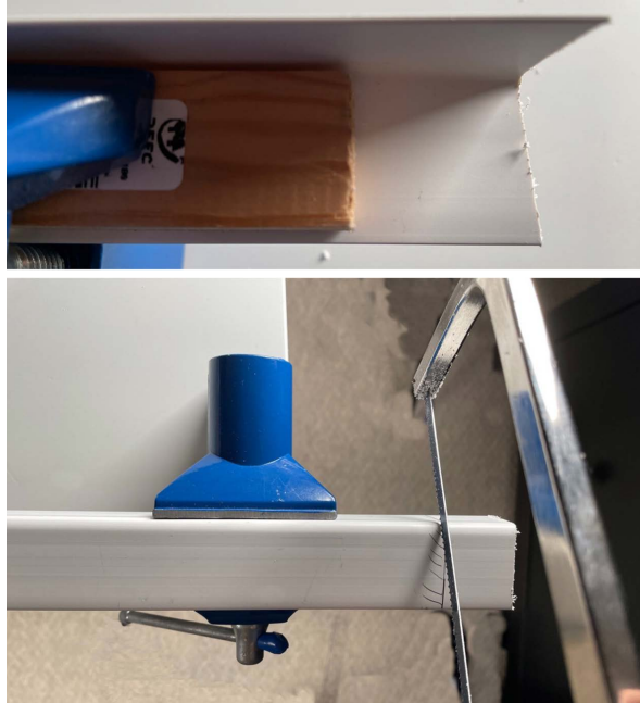
Figure 7.15 – Cutting the sensor brackets
