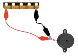
**Note:** Do not attempt this with an active Piezo buzzer - such buzzers are only able to play a single tone.
