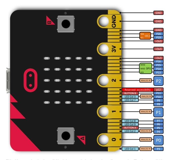
This table summarises the pins available, their types and what they are internally connected to. The pins are available as attributes on the microbit module: microbit.pin0 - microbit.pin20.
