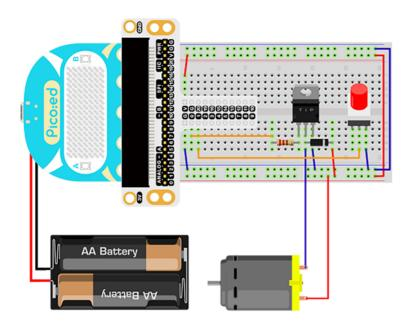
The drive current of the IO port of the <u>Pico:ed</u> is very weak, not enough to directly drive the motor. At this time, we need to use a triode to amplify the current of the IO signal. The circuit diagram of using a triode to amplify the signal current of the IO port is very similar to the circuit diagram of driving the buzzer in the previous lesson. The only difference is that one is added at both ends of the motor. diode. This diode is called a freewheeling diode in this circuit.
