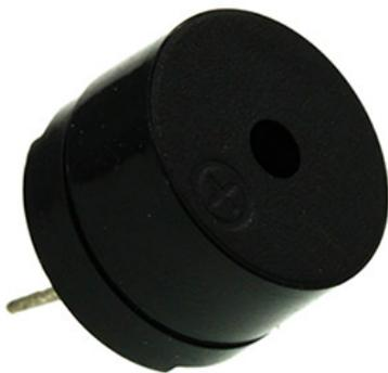
Here's the working principle of active buzzer: Because active buzzer has integrated amplify sampling circuit and resonance system, when DC power input passes through active buzzer, it will make resonance device generate sound signal. We can see the schematic diagram below for the working principle of active buzzer:
