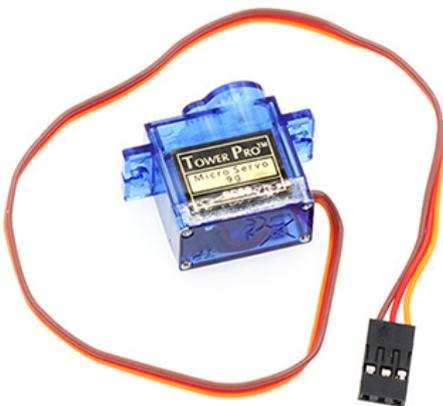
There are many specifications for servos, but all servos have three external wires, which are distinguished by three colors: brown, red, and orange (different brands may have slightly different colors), brown is the ground wire, and red is the positive pole of the power supply line, orange is the signal line.
