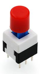
*Note:* This self-locking switch consists of two sets of pole double throw switches, only one of which is used in this test, so the common pins of one of them are cut off.
