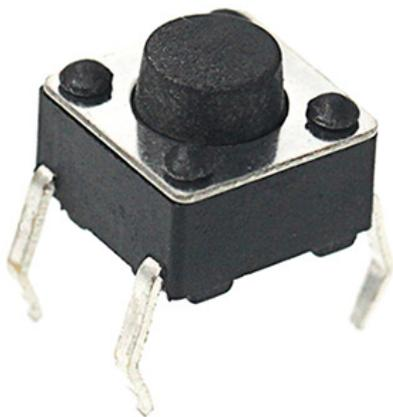
Momentary push button switches have 4 pins. The 4 pins can be divided into 2 groups: pin 1 shorted to pin 2, pin 3 shorted to pin 4.
