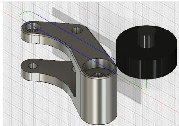
**Bore larger holes:** Create a bore operation to machine the counterbores on two holes.
