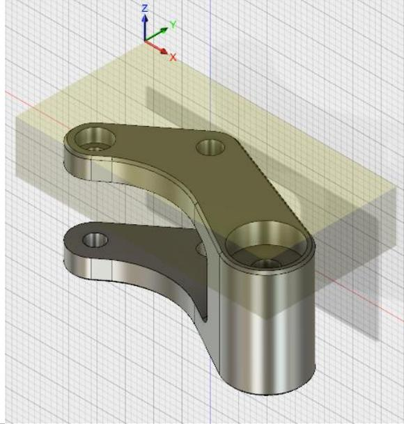
**Face operation:** Create a face operation and use the same face mill as in the previous face operation.
