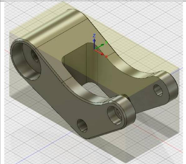
**Create Setup 3:** Create the second setup and stock to continue machining the part.
