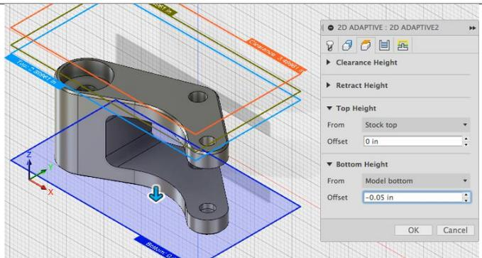
Machining past the part during roughing gives you a nice finish/transition when you face the backside.
