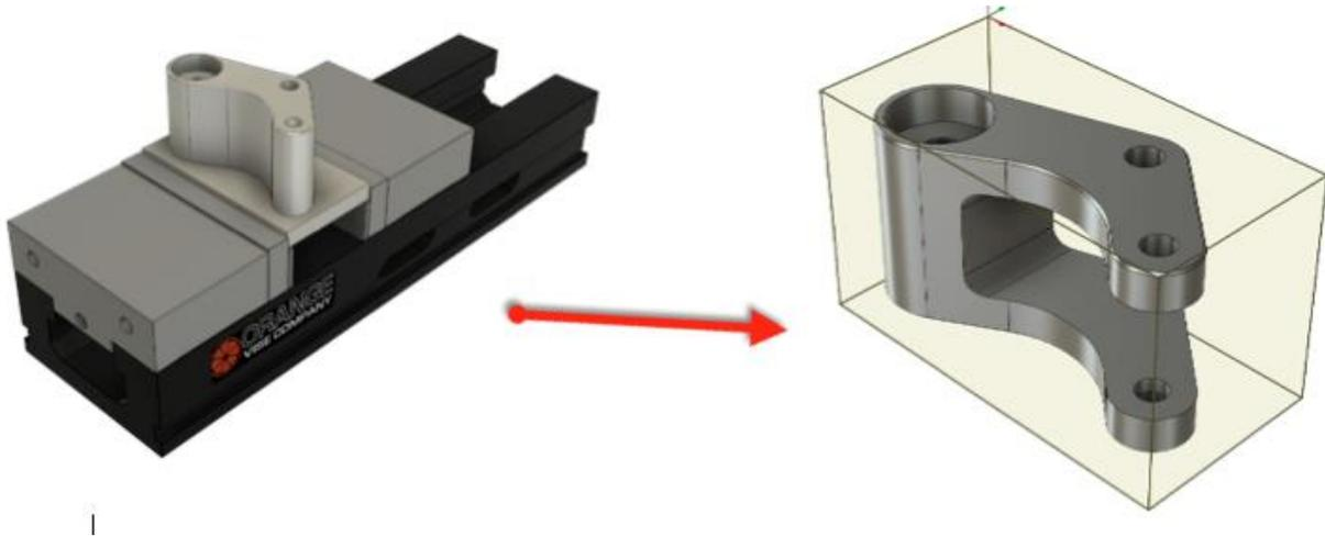
**Create the first setup:** In this section, you go to the CAM workspace, create a setup, then set your stock.
