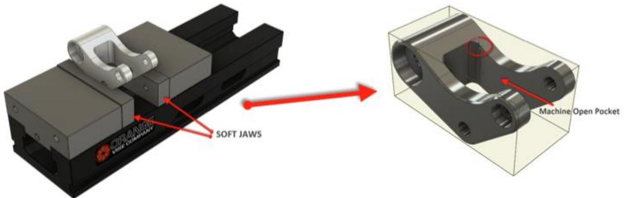
**Create Setup 3:** Create the second setup and stock to continue machining the part.
