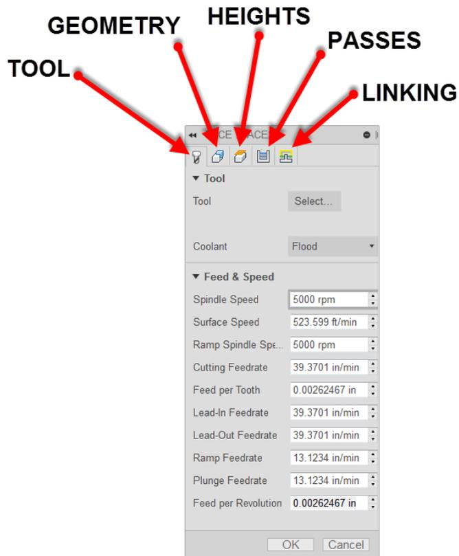
**Tool:** Defines the tool being used as well as the feeds and speeds.
