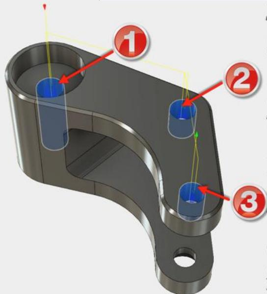
Step 6 – Simulate the setup
