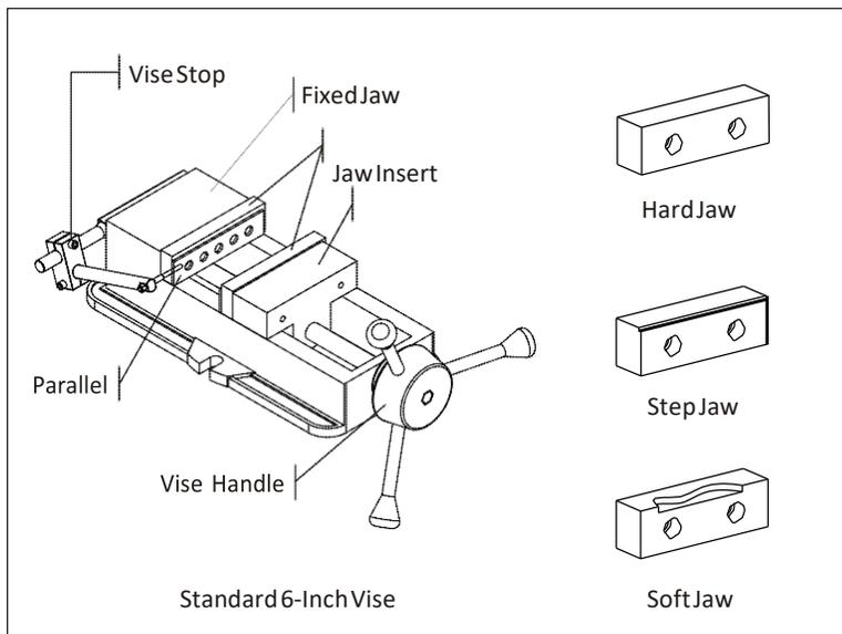
The **Fixed Jaw** remains stationary. The **Moving Jaw** opens when the **Vise Handle** is turned. It is a good practice to remove the vise handle after the jaws are closed and before running the program. This is done by sliding the handle off.
