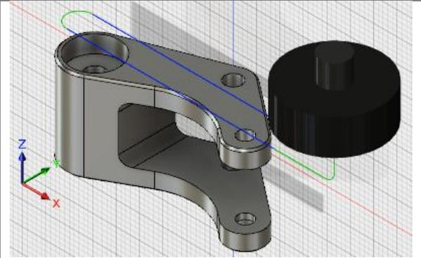
**Adaptive Clearing:** Create an adaptive clearing operation to remove material around the outside of your design.
