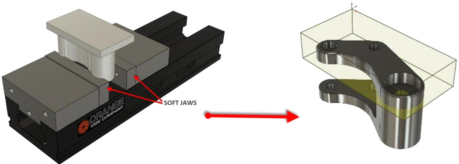
**Create Setup 2:** Create the second setup and stock to continue machining the part.
