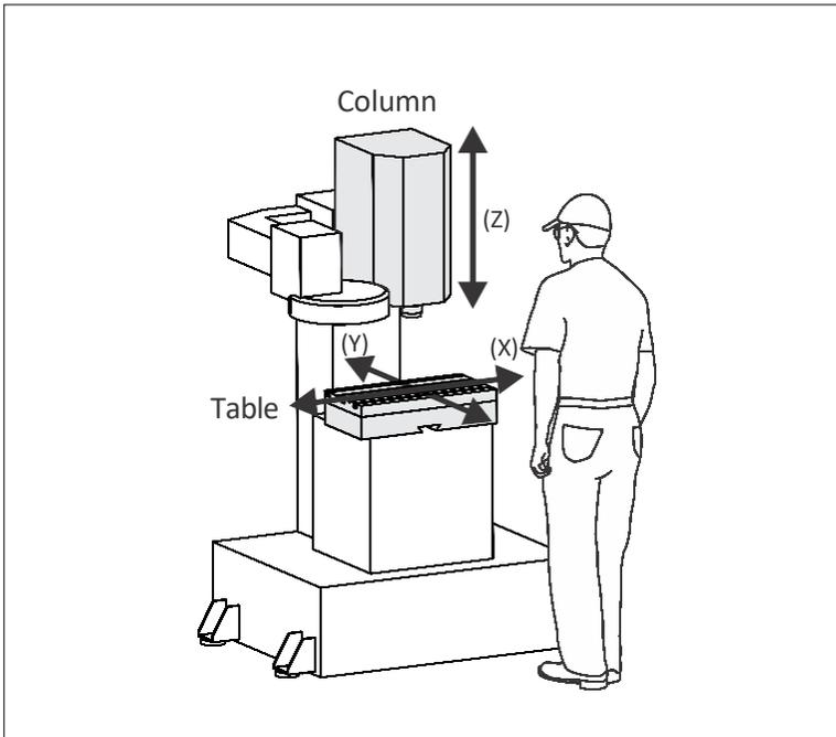
CNC machines use a 3D Cartesian coordinate system. Figure 10 shows a typical.
