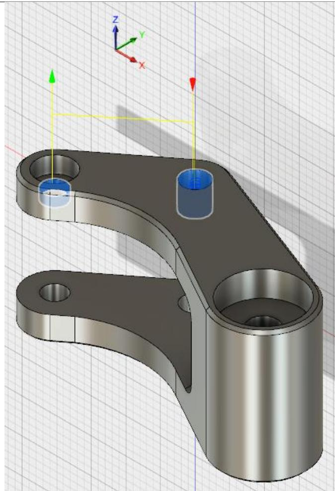
**Chamfer edge:** Finish this setup by chamfering the edge of the part.
