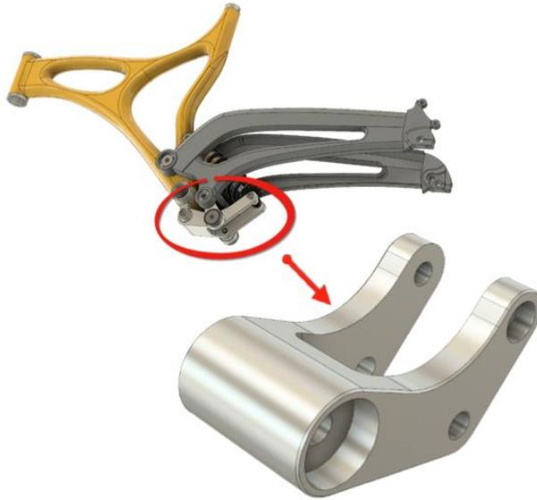
Using 2.5 Axis Functionality, we will begin with a block of Aluminum Stock mounted in a Vise (see Figure 1), and will create three (3) 'job setups' that will be required to machine the Rocker Arm.
