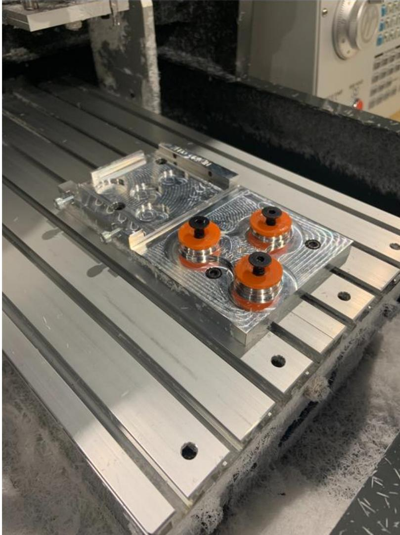
1. With this project, we will use the paper shim method for qualifying a Work Offset fixture position.
