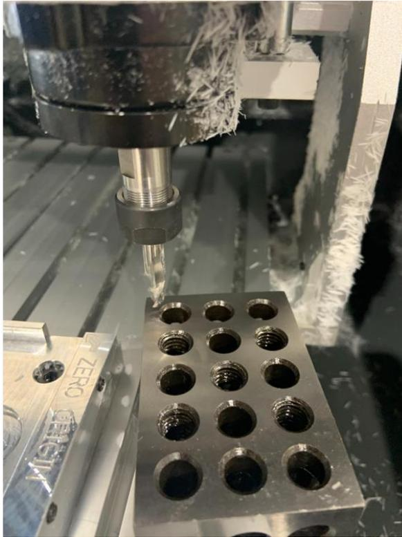
4. Make sure to move the 1-2-3 block out of the way slightly so that you can jog the tool down lower than the 1-2-3 block on purpose. Do not jog the tool into the 1-2-3 block causing damage.
