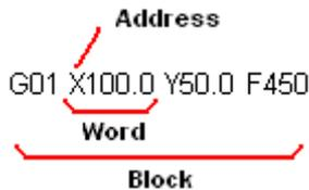
G01 X100.0 Y50.0 F450 is a block. It tells the tool to move along a straight line to X100.0 Y50.0 at a feed rate of 450 mm/min.
