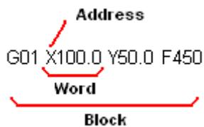
G01 X100.0 Z50.0 F0.2 is a block. It tells the tool to move along a straight line to X100.0 Z50.0 at a feed rate of 0.2 mm/revolution.
