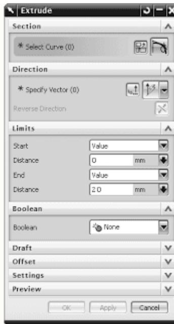
You will be prompted to select the planar face to sketch or the section geometry to be extruded. If you select the sketch at this stage, the preview of the extruded feature created using the default values will be displayed on the screen. If you select the sketch plane, the Sketcher environment will be invoked. Draw the sketch and exit the Sketcher environment; the preview of the extruded feature will be displayed in the Modeling environment.
