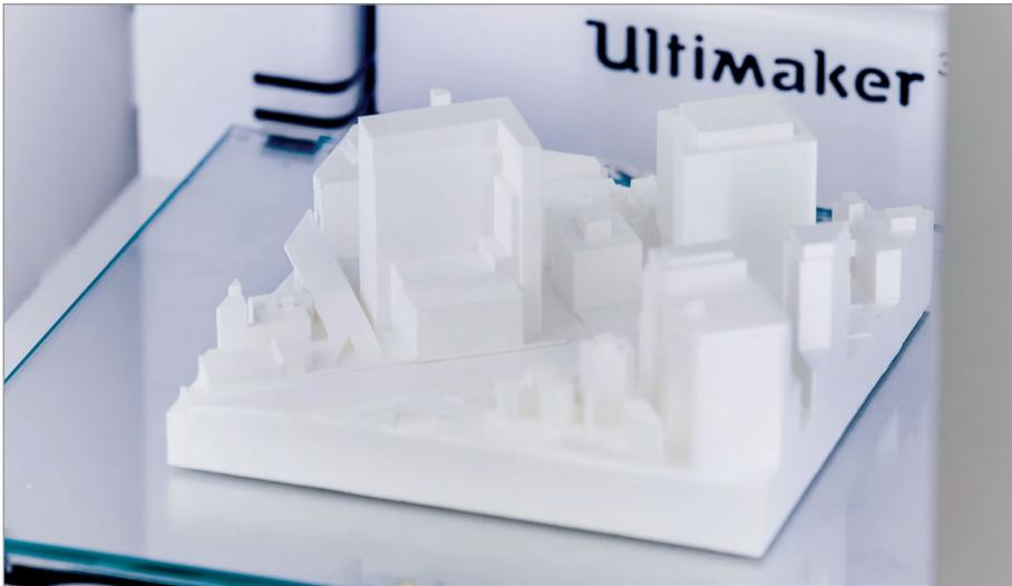
**FIGURE 2.6** – Architectural model printed with an Ultimaker 3D printer. Svitlana Lozova.
