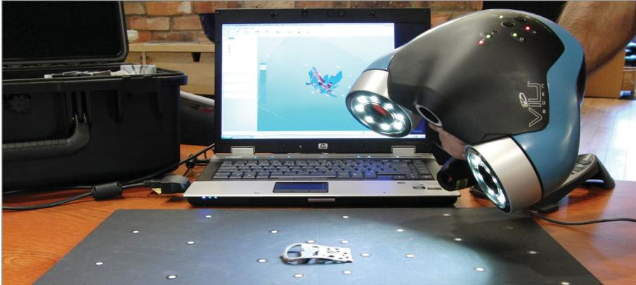
**FIGURE 2.4** – Making a 3D model of a Viking belt buckle using a handheld VIUScan 3D laser scanner. As the device uses a laser scanner to create a 3D model, it also uses a camera to accurately texture map the object. This 3D file is the result of a project in which a 1000-year-old Viking belt buckle was laser scanned and 3D printed to achieve a copy of the unique archaeological artifact. Creative Tools.
