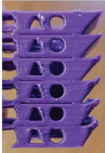
**FIGURE 10.6** – Small features become overheated and deformed. Jonathan Torta.
