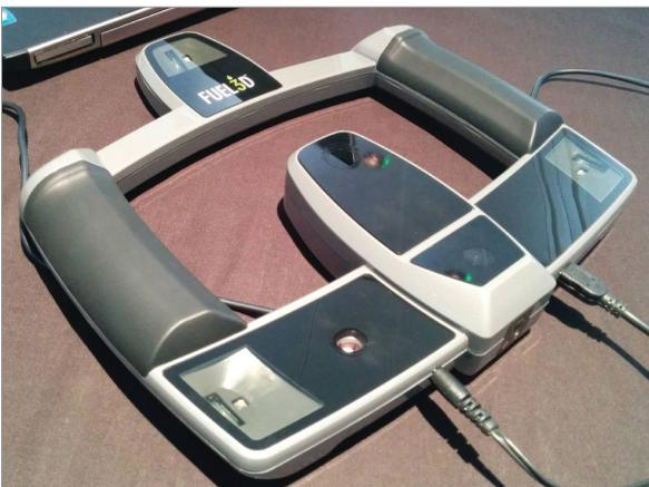
FIGURE 8.1 – Fuel3D portable 3D scanner. Creative Tools.
