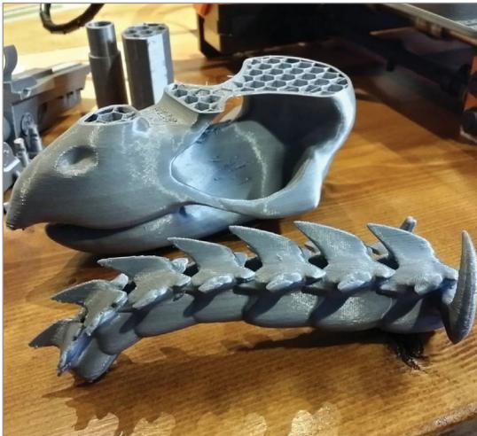
**FIGURE 4.21** – 3D printed statue that was printed in parts. Lucas Phillips.
