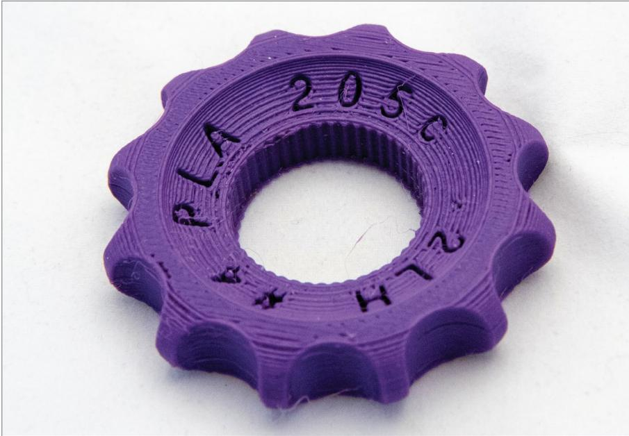
**FIGURE 11.8** – Example of a Maker Coin, with filament and temperature information embossed on it. Jonathan Torta.
