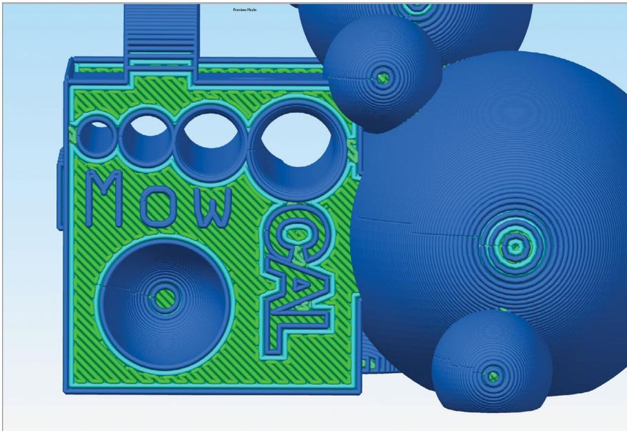
**FIGURE 12.17** – Sliced with words “flat” (x/y axis) with a 0.4 mm nozzle. Jonathan Torta.
