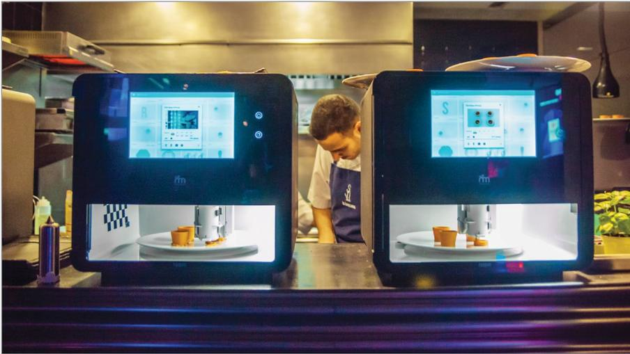
**FIGURE 2.12** – Foodini 3D food printer being used in a restaurant. Natural Machines.
