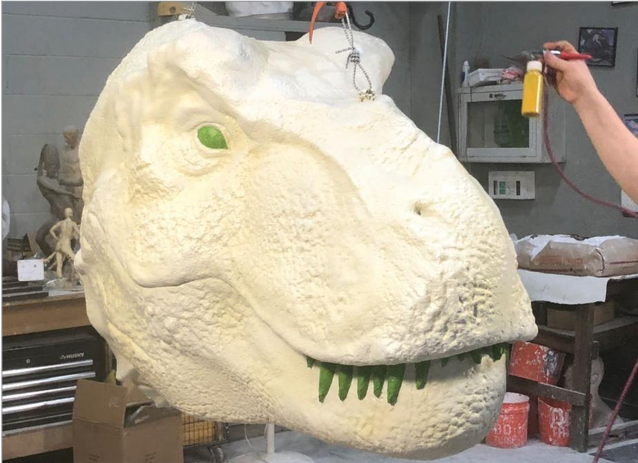
**FIGURE 13.7** - The preparation and painting process of a 3D printed dinosaur head. Nina Buccacio.
