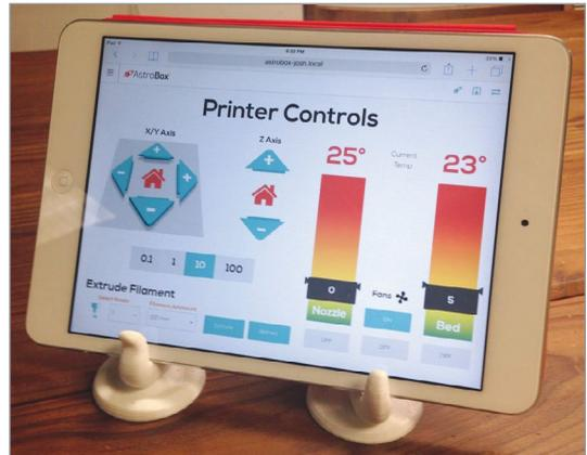
**FIGURE 7.16** – AstroPrint interface on a tablet while remotely managing a 3D Printer. JayLoerns
