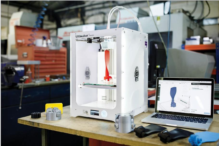
**FIGURE 1.1** – A number of 3D printed functional prototypes sliced in Ultimaker Cura and 3D printed on Ultimaker 3 Extended with PLA and water-soluble PVA. Svitlana Lozova.
