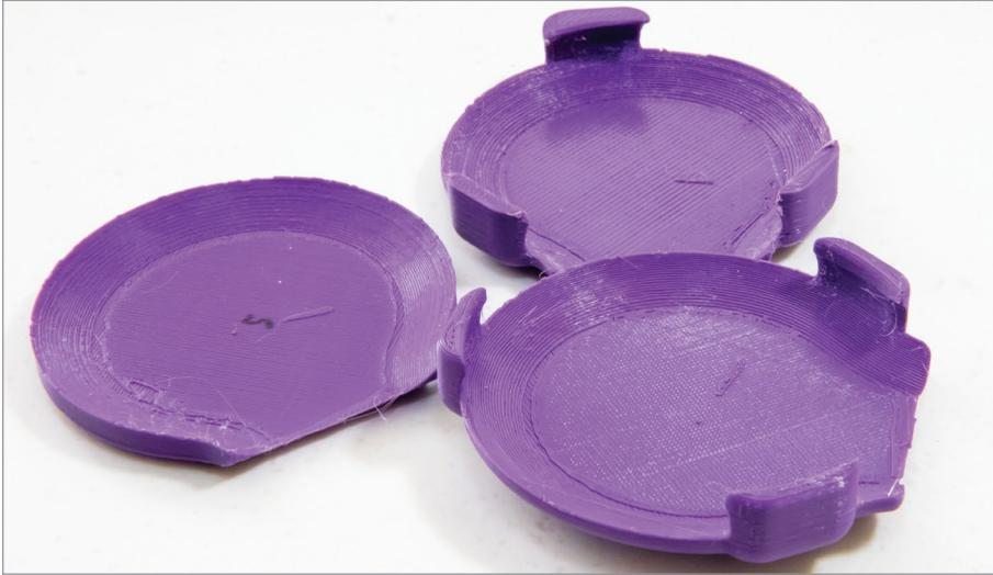
**FIGURE 4.7** – Prototypes of the 3D printed mounting plates. Jonathan Torta.
