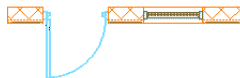
Plan display representations for wall, door, and window shown in 2D from a plan view direction
