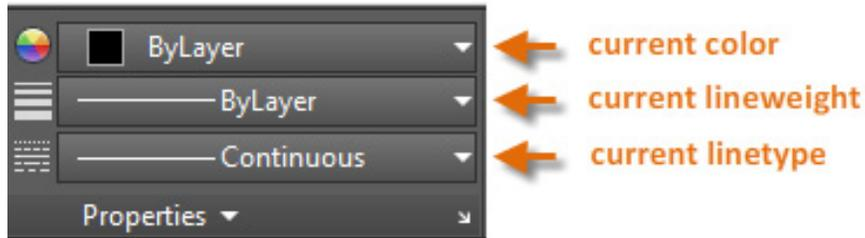
The Properties panel works the same way as the Properties palette. When you select an object, the current property settings are replaced by the properties assigned to the selected object, and you can use this panel to easily change the properties of one or more selected objects.
