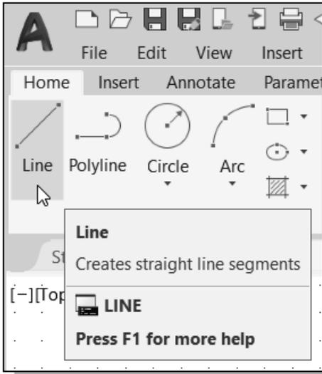
1. Select the **Line** command icon in the *Draw* toolbar. In the command prompt area, near the bottom of the AutoCAD graphics window, the message “*\_line Specify first point:*” is displayed. AutoCAD expects us to identify the starting location of a straight line.
