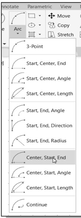
1. Click the down-arrow icon of the **Arc** command in the *Draw* toolbar to display the different Arc construction options.
