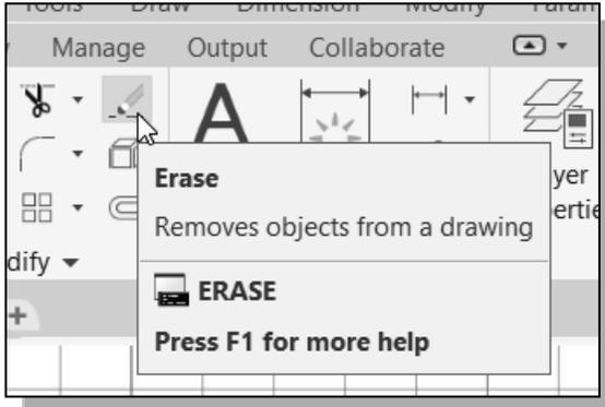
1. Pick **Erase** in the *Modify* toolbar. (The icon is a picture of an eraser at the end of a pencil.) The message “*Select objects*” is displayed in the command prompt area and AutoCAD awaits us to select the objects to erase.
