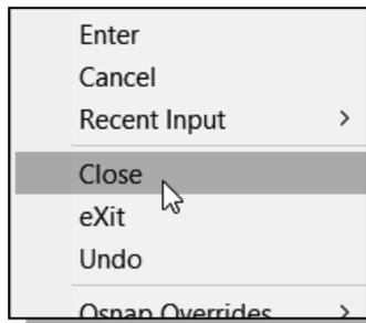
15. For the last segment of the sketch, we can use the **Close** option to connect back to the starting point. Inside the graphics window, **right-mouse-click** and a *pop-up menu* appears on the screen.
