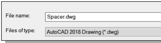
3. Click **Save** in the *Save Drawing As* dialog box to accept the selections and save the file. Note the default file type is DWG, which is the standard AutoCAD drawing format.
