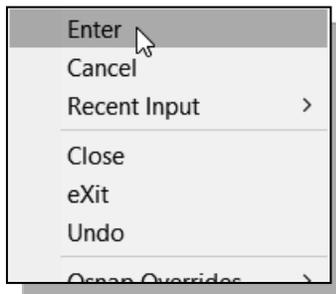
9. To end the line command, we can either hit the [Enter] key on the keyboard or use the **Enter** option, **right-mouse-click** and a *pop-up menu* appears on the screen.
