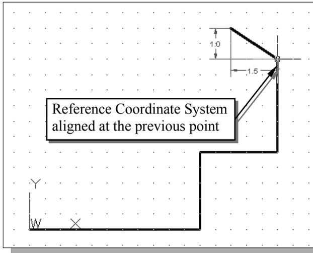
13. Using the *relative rectangular coordinates entry method* to create the next line, we can imagine a *reference coordinate system* aligned at the previous point. Coordinates are measured along the two reference axes.
