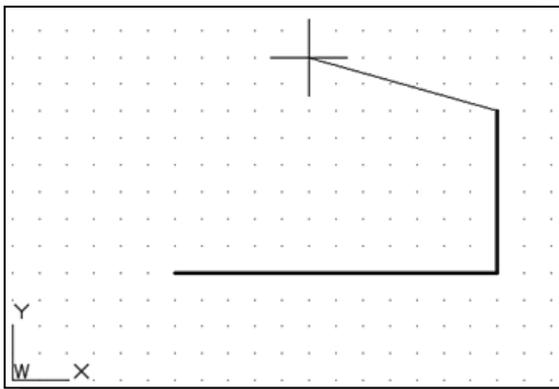
4. Next, create a vertical line by using the *relative polar coordinates entry method*, relative to the last point we specified: **@3<90 [ENTER]**
