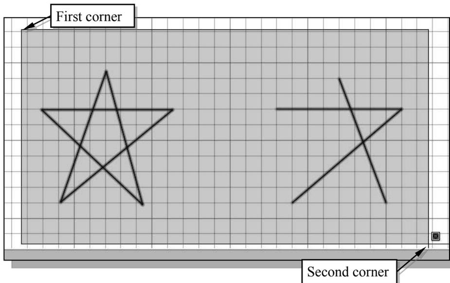
4. Move the cursor toward the right and below the entities, and then left-mouse-click to enclose all the entities inside the **selection window**. Notice all entities that are inside the window are selected. (Note the **enclosed window selection** direction is from **top left** to **bottom right**.)
