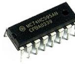
Examine the diagram carefully. Connect the 3.3v to the top rail of your Breadboard and the Ground to the bottom. The chip has a small dimple on one end, this dimple goes to the left. Pin 1 is below the dimple, Pin 8 at bottom right, Pin 9 at top right
