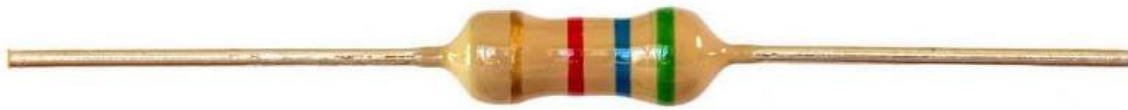
A resistor limits the amount of current that flows through a wire
