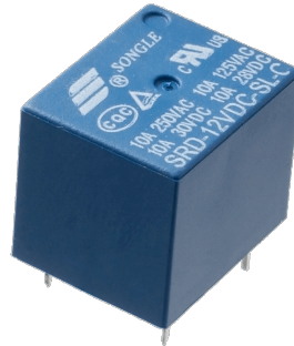
A relay is used to drive large loads from your Arduino
