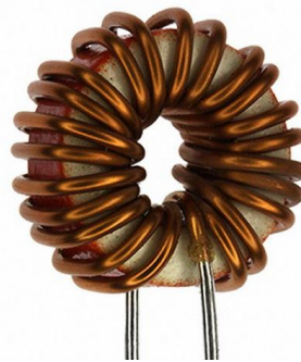
A coil can be used as a filter.
