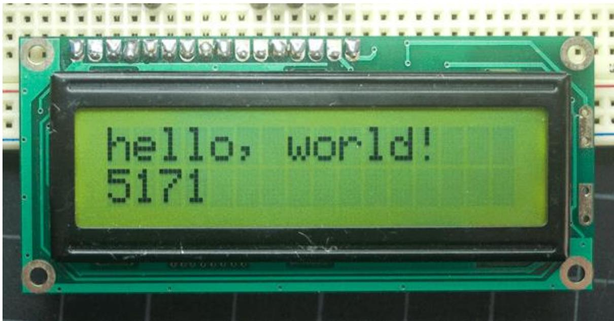
Fig. 21 Output of the sketch in 16x2 LCD
