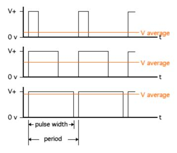
By using Arduino's analogWrite(pin, value) function we can vary the value of the duty cycle of pin's output. Note that the pin must be put into output mode and the value must be between 0 (0V) and 255 (5V). Any value in between will simulate a proportional intermediate analog output.
