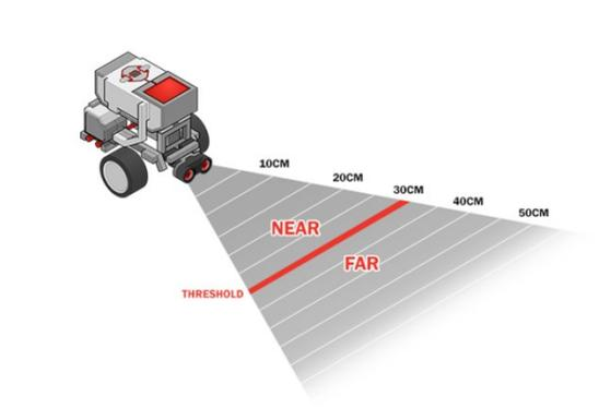
This way, the Wait Block does not have to worry about the difference between an object at 29cm and an object at 30cm; it only has to worry about whether the value is above or below the Threshold.
