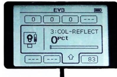
"COL-REFLECT" means the sensor is reading amount of colored light being reflected.
