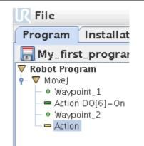
Continue programming we wish to control the same output after the robot has moved to the Waypoint\_2. Press the Waypoint\_2 and go to "Structure" tab and pick one more I/O action.
