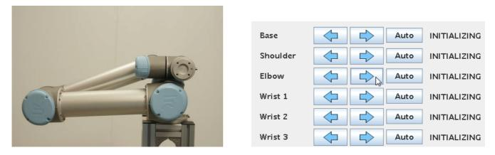
In this position we need to make sure the robot is moving "upwards" so it is not crashing into itself. If it crashes into itself it will stop with a safety stop, but the robot could be slightly scratched and we want to avoid that especially when it is new.
