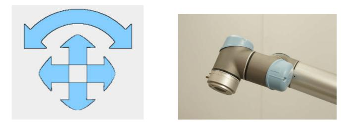
On the left side on the Move Screen below the Up and Down arrow keys are a set of arrow keys that can move the robot in relation to the tool head position.
