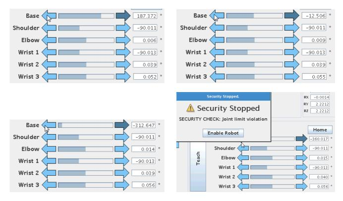
The same error messages occur when you turn the robot joint 720 degrees all the way to the other side. Press "Enable Robot" to acknowledge the error messages. Notice how this part of the arrow bars handles each joint individually.
