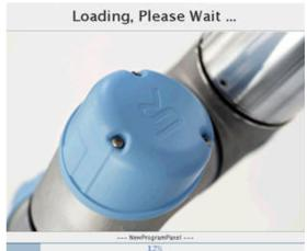
During boot you will see various screens loading and checks – this is normal and it takes 1 - 2 minutes to boot. You will also hear the fans turn in the controller box.
