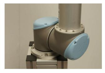
Now the robot is fully stretched is a nice position to start moving each joint to see how the robot moves. Start with the base joint and press the Arrow bar left or right and see how only the base joint moves.
