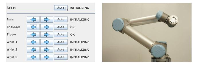
Now the robot is already quite good up and free so for the last 4 joints we will use a faster method. Press the "Auto" button on top of all joints where it says "Robot".
