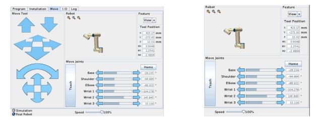
The screen has several functions, but the main purpose is to move the robot around in its space during programming and to get a report where the joints are located which are shown on the degree position of each joint or above by the X - Y and Z position indicator.
