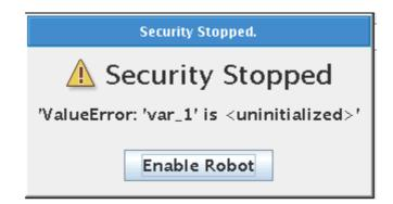
If you get this error messages it is because we need to tell the Robot – what should the variable "var\_1" be when we start the program. This is uncertain for the robot if we have not explicit set the variable before the program execution.
