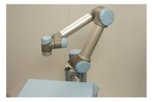
The robot runs this program beautifully without any error messages in MoveJ mode because it is allowed to take a bended route from Waypoint\_1 and Waypoint\_2 UNIVERSAL ROBOTS
