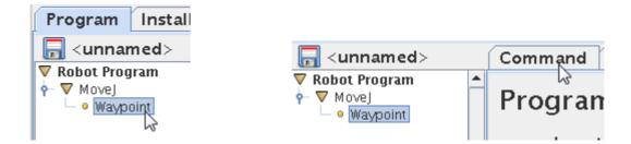
We need to define each Waypoint we insert into out program. Point and press on the Waypoint we want to define – in this case there is only one because we just started programming. Press the "Command" tab.
