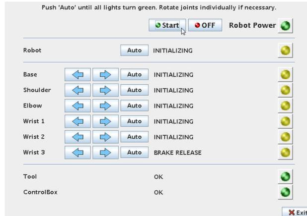
After a short time you will see the “BRAKE RELEASE” go to “INITIALIZING” status for all joints. In some firmware version you will also shortly see the messages “BOOTING” for the joints
