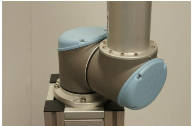
Now the robot is fully stretched is a nice position to start moving each joint to see how the robot moves. Start with the base joint and press the Arrow bar left or right and see how only the base joint moves.
