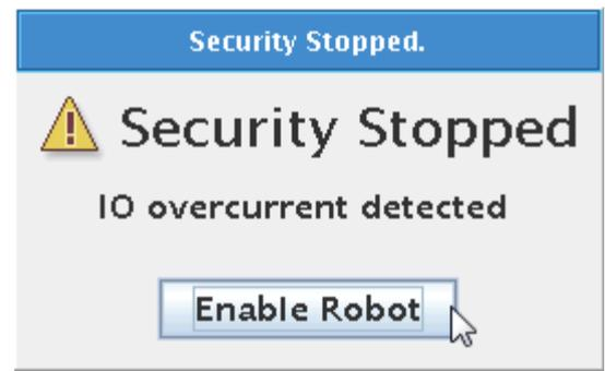
The output is not current limited, but if the output is short circuited it will result in a security stop and error messages because of over current detected on an output.
