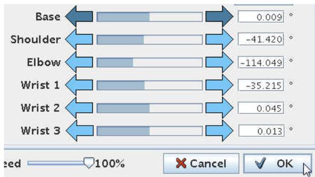
While we were manually manipulating the robot around with our hand we had the Move Screen on the monitor. Press the “OK” button in the lower right corner of the Move Screen which takes you back to the Program window.
