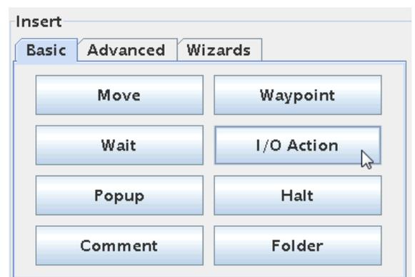
Since we already have to program lines then we need to decide where we want to have out action. In this case we want it in between the two Waypoints so we place the cursor by pressing the first Waypoint. Press the “Structure” tab. This time choose an “I/O Action”.
