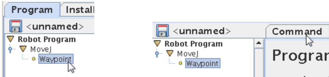
We need to define each Waypoint we insert into our program. Point and press on the Waypoint we want to define – in this case there is only one because we just started programming. Press the “Command” tab.
