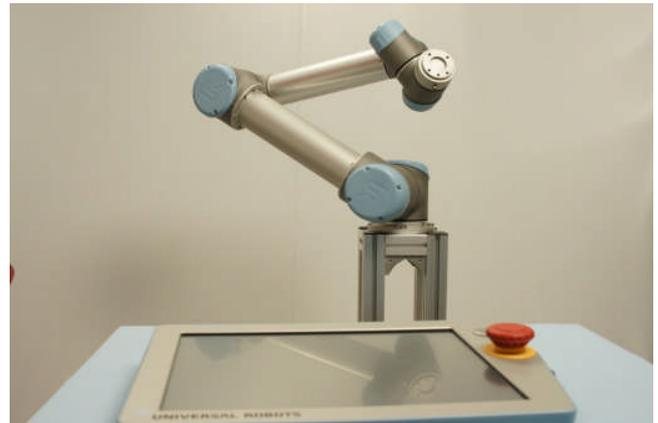
All the joints on the monitor reports “OK” and notice how all the lamps turned green. The robot is now initialized and ready to be programmed or load a program if we already have made a program before.
