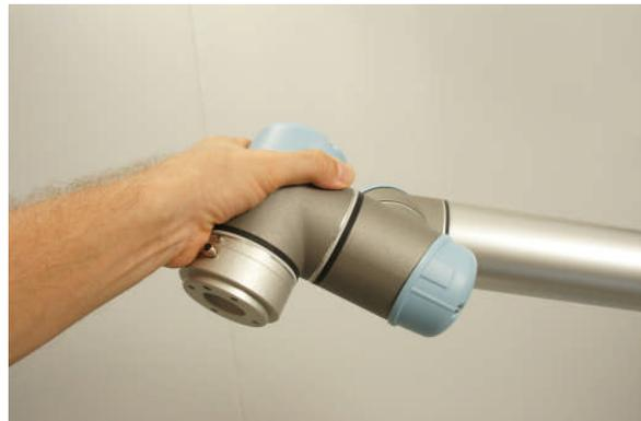
Press and keep pressing the black button on the back of the monitor and grab the robot and start moving into your desired position.
