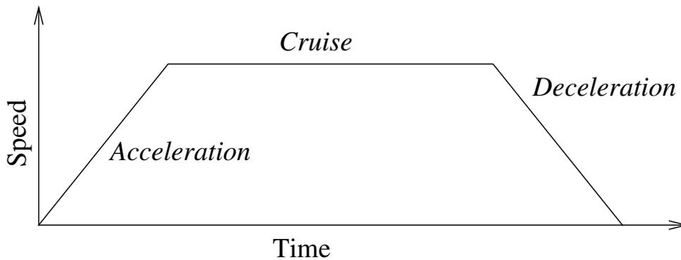
Figure 14.1: Speed profile for a motion. The curve is divided into three segments: *acceleration*, *cruise* and *deceleration*. The level of the *cruise* phase is given by the speed setting of the motion, while the steepness of the *acceleration* and *deceleration* phases is given by the acceleration parameter.
