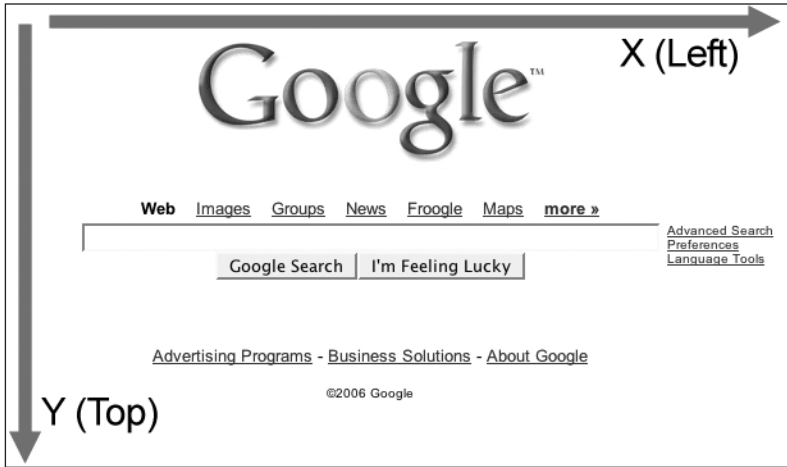
Figure 7-1. An example of the coordinate system on a web page using CSS
