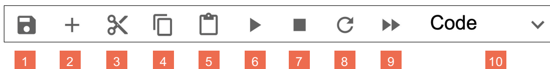
Figure 6. Jupyter Notebook top bar: (1) save Notebook, (2) add cell, (3) cut cell, (4) copy cell, (5) paste cell, (6) run cell, (7) interrupt kernel, (8) restart kernel, (9) restart kernel and run whole Notebook, and (10) define cell as code or markdown.
